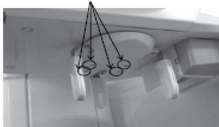
Phillips pan-head machine screw (M4 x L8 with spring and flat washers)
