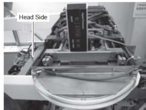
Fig. ③ -36: Checking Levelness in Horizontal (Left-Right) Direction 3
